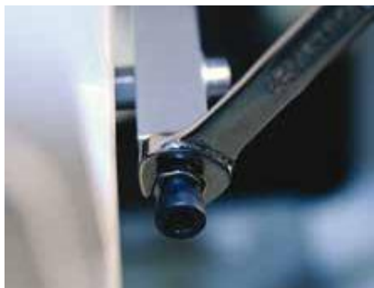
Figure A5: Adjusting the right stop
