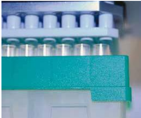
Figure A3: Non-aligned nozzles (exaggerated view)
