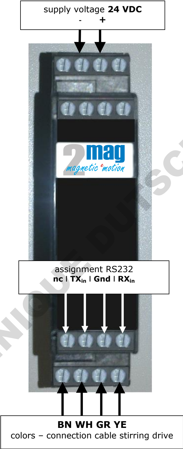
Image 9: Pin-assignment of MIXcontrol eco DINrail RS232
