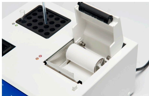
Fig. 2: Paper in V-shaped roller supports
