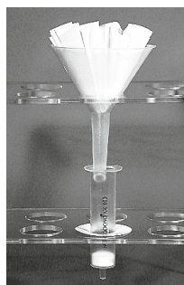
Figure 1 Correct use of the NucleoBond® Folded Filter, NucleoBond® Column placed in a Plastic Washer
