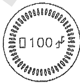
VIEW ON BASE SHOWING EMBOSSED MARKING STANDING AREA EMBOSSED WITH RADIAL BAR STIPPLE
