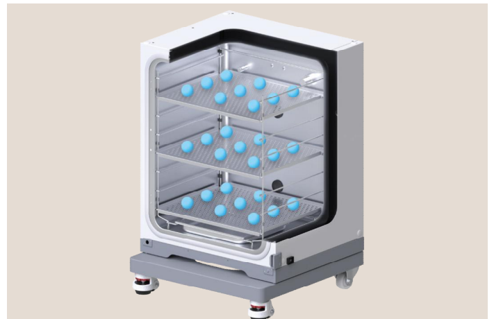
Fig. 1: Measurement set-up according to DIN 12880:2007-05 – 27 temperature probes placed at different locations on three shelves inside the CO 2 incubator
