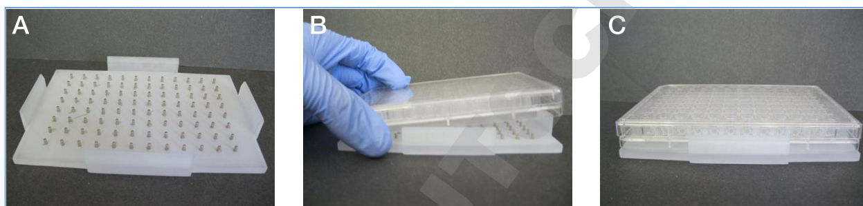
Figure 4: Take the spheroid drive (a) and place a cell-repellent 96-well plate (b) atop the spheroid drive to print the cells into a spheroid (c).
