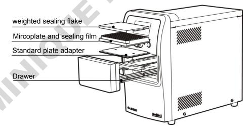
2.1 Press "**PLATE In/Out**" key, and pull the drawer, Then put in the standard plate adapter, micro-plate and sealing film and the weighted sealing flake in turn.
