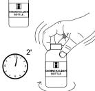
• Flip open the top of the Demineralizer Bottle cap. By gently squeezing the bottle, add demineralized water to the other vial up to the 20 mL mark. Replace the cap and shake to mix.
