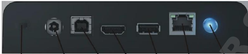
Slot for Kensington lock Power Supply USB B HDMI USB A Ethernet Power On/Off
