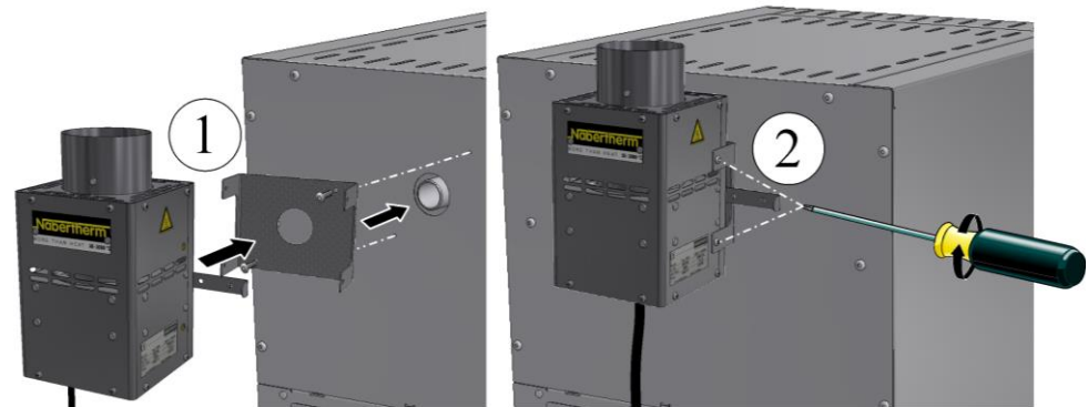
Fig. 22: Vent with fan (similar to picture)
