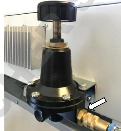
Figure 12: Compressed air connection on the pressure regulator
