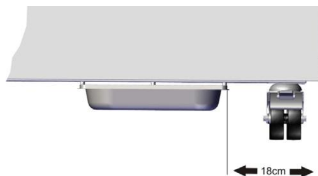
Figure 17: Positioning the condensate collection pan (front view)
