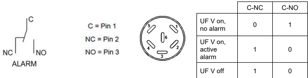
Figure 24: Zero-voltage contacts circuit diagram and pin allocation of DIN socket (9)
