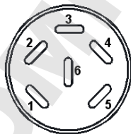
Figure 20: Pin allocation of DIN socket (3) for option analog outputs
