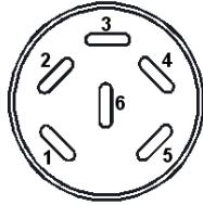
Figure 21: Pin configuration of the DIN socket (6)
