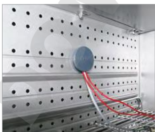
Access port with silicone plug
