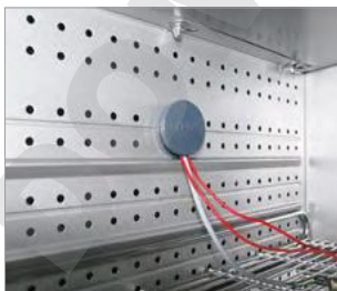
Access port with silicone plug
