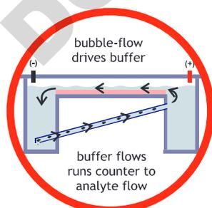
Galileo automatic buffer recirculation reduces detrimental ion and pH gradients in your buffer, providing even migration for long running gels.
