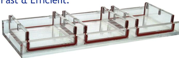
Also available is the RapidCast™ gel casting frame which allows casting up to 3 gels at once, even while the mini-gel unit is in use.
