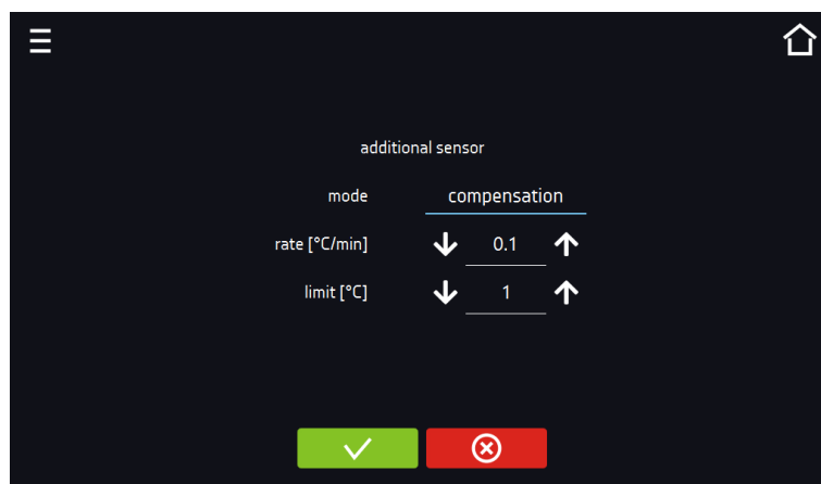
Figure 95 Temperature measurement settings with an additional sensor
