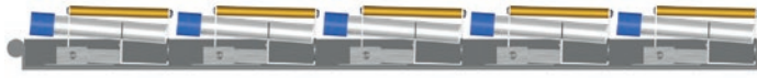
Hettich-Rack L with tubes of length 120 mm at an angle of inclination of 5°
