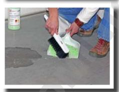
themsolute SOrb embeds the absorbed chemicals into its gel structure and resulting in an almost dry surface.
