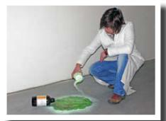
chem<sup>solute®</sup> **SOT**b should be sprinkled equally and extensive on surface of spilt chemicals or oil.
