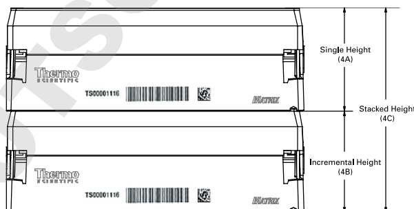
▲ Figure 4: Stacked Rack View
