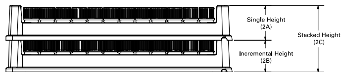
▲ Figure 7: Stacked Tray View
