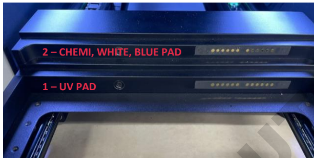
Figure 2. Tray levels. Bottom tray (numbered 1) for UV PAD and Top tray (numbered 2) for Chemi, White and Blue PAD
