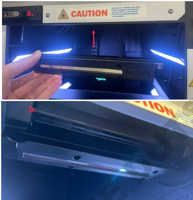
Figure 9. a. ChromaScan Excitation Source. Red arrow indicates location of ChromaScan wheel b. Final position of ChromaScan Excitation source on the mechanical wheel
