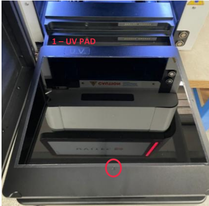
Figure 3. UV tag, chip and arrow facing the inside of the system. Proceed to slide UV
