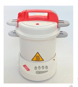
434000 offers multiple benefits for users. The Autoclave is 9 litre capacity, light weight, with a 126 degrees C sterilising temperature. The internal furniture consists of a basket as standard, however can also be supplied with cassette holders for instruments.
