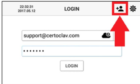
When the touch screen is switched on, the login window appears. To create a new user, press the “plus”-icon in the top right corner of the screen.
