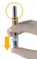
Figure 12 Lubricate the internal part of the piston
