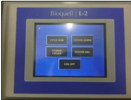
9. Press 'STORED CYCLES' to edit the settings parameter
