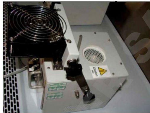
4. Point the vaporizer fan towards front grille:
