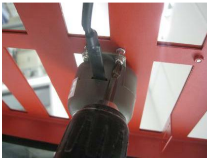
Figure 1.10. Remove doughnut sensor housing
