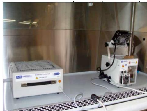
2. Place the internet catalyst and vaporizer on tray
