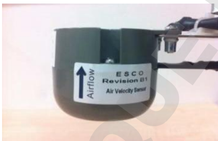
Figure 1.11. Airflow sensor direction
