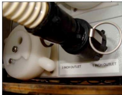
8. Connect 1" hose to 1" outlet on external catalyst:
