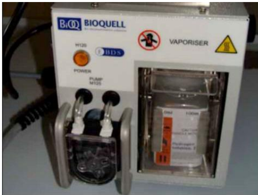
3. Insert the hydrogen peroxide bottle:
