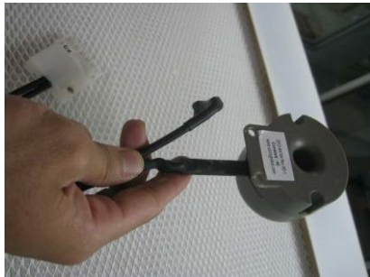
Figure 1.9. Remove Temperature sensor
