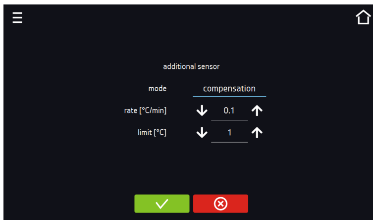
Figure 95 Temperature measurement settings with an additional sensor
