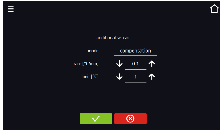
Figure 95 Temperature measurement settings with an additional sensor
