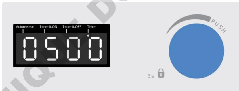
After the timer has elapsed, the stirring will be stopped and the display will show *End*.
