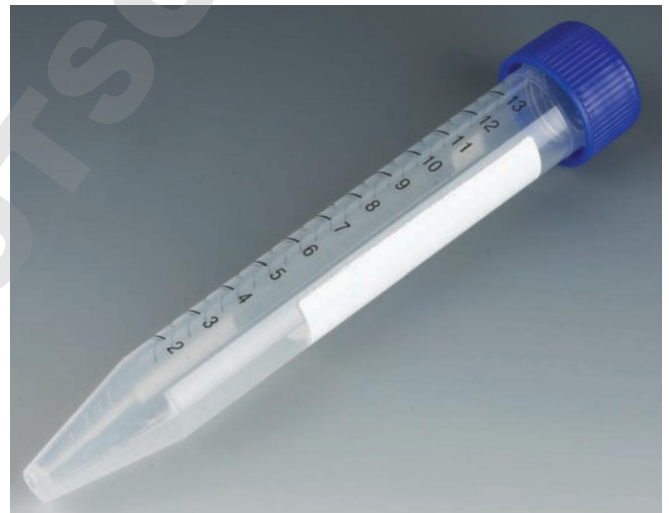
15mL polypropylene centrifuge tube
