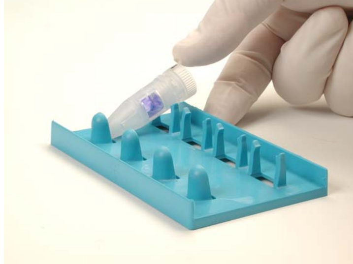
Figure 1: Insertion of the GeBAflex-tube in the provided supporting tray. The arrow on the cap is pointing upwards.
