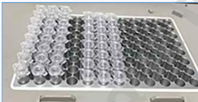
Figure 8: Fit of 0.1 ml low profile and 0.2 ml standard PCR tubes in an ABI 9700 PCR Thermal Cycler. The adjustable lid of the cycler allows the use of 0.1 ml low profile tubes. The reduced height of the low profile tubes minimises the gap between heated lid and reaction mix resulting in lower evaporation and higher accuracy of the polymerase chain reaction
