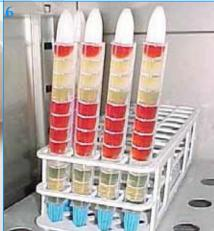
Replace both caps. Incubate at 35 to 37° C for 18 to 24 hours with EnteroPluri-*Test* lying on its flat surface or in an upright position. Allow for air circulation between incubated tubes.
