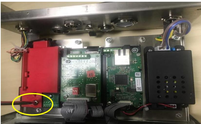
4. Pull the protruding part of the sealing cover a little forward to release it.
