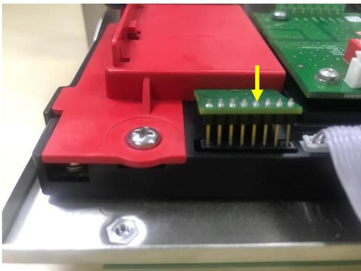
6. Use a screwdriver to tighten the screw and make sure the Alibi memory board is installed properly.
