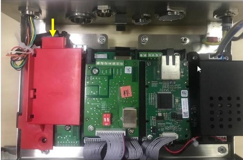
5. Remove the sealing cover and then unplug the white load cell connectors.
