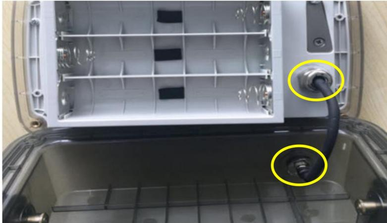
3. Open the front housing by removing the 12 Phillips head screws.
