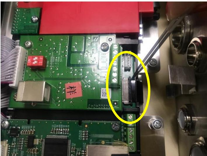
4. Make sure the whole FPC socket are pushed in and the button cable is attached to it firmly.
