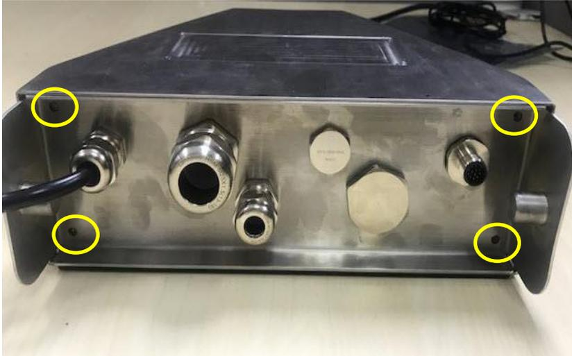
2. Open the housing by carefully pulling the bottom housing backward.
