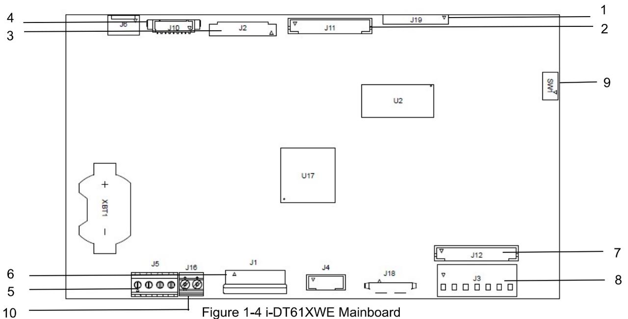
Figure 1-4 i-DT61XWE Mainboard
