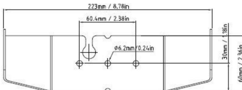
Figure 2-8 Dimensions du support de montage i-DT61PW
