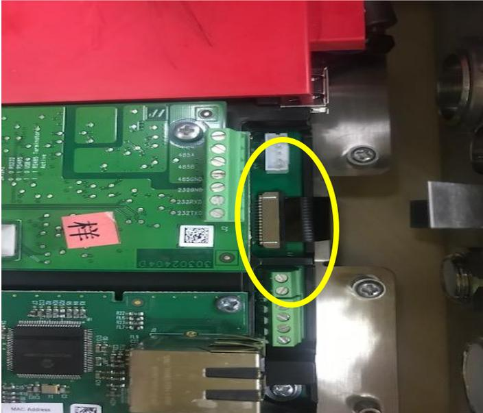
5. Repeat the previous step 7 to push in the bottom of the terminal and tighten all the screws.
