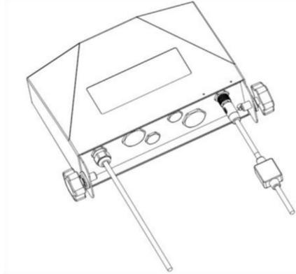
Figure 5-5. Connecting cable with connector and memory module
