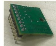
5. Insert the Alibi memory board into the slot as shown below. Please make sure the pins are properly inserted.
