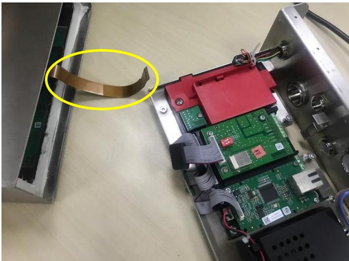
1. When you finish to install the Albi memory board, pass the button cable through the bottom of the meter.
