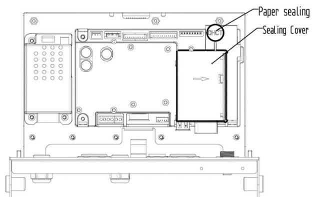
Figure 5-3. i-DT61PW Wire Sealing
