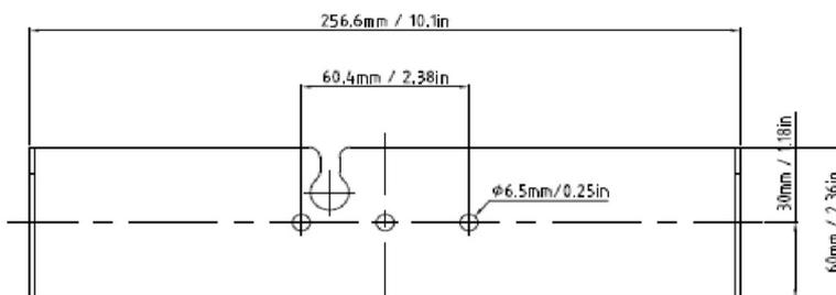
Figure 2-9 Dimensions du support de montage i-DT61XWE
