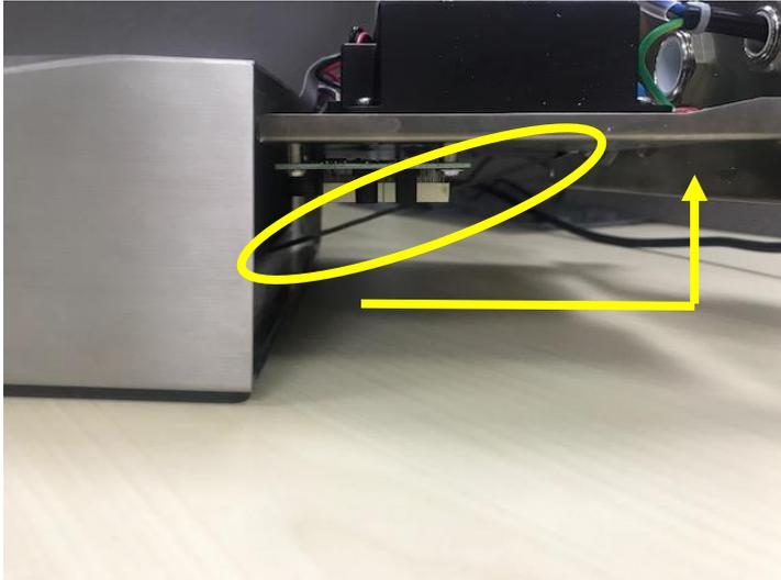
2. And pull it under the FPC socket. Push the button cable further under the FPC socket so that the cable is firmly attached.
