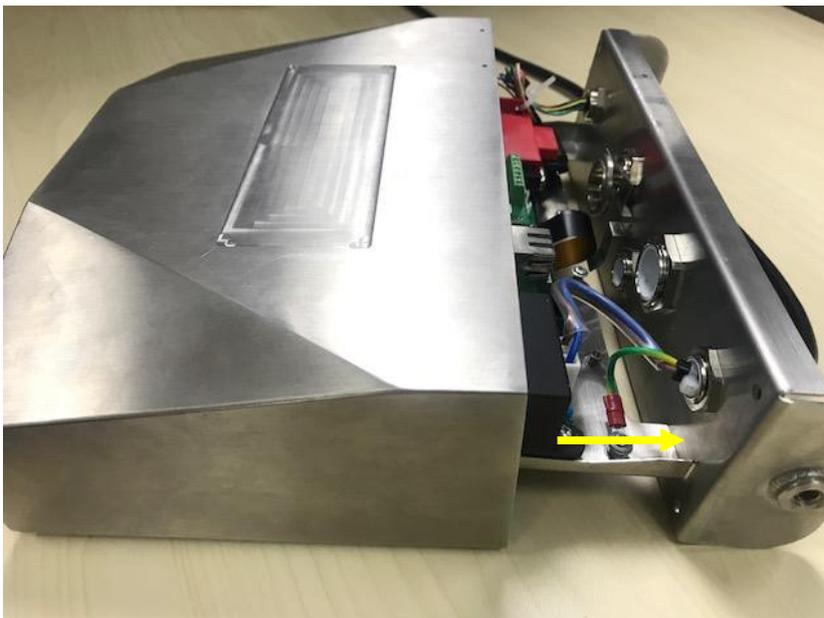
3. Once all connections are made, re-attach the bottom housing.
