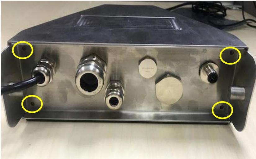
2. Pull out the bottom of the terminal.
