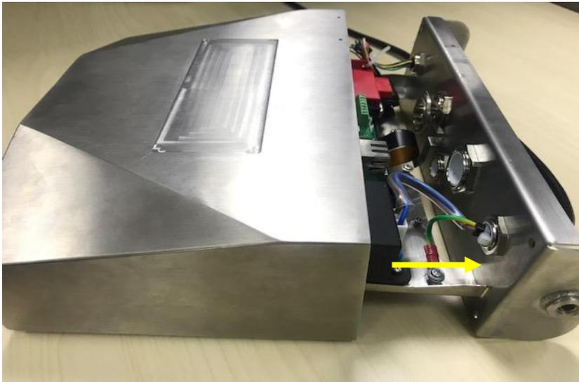
3. Use a screw driver to unscrew the sealing cover.
