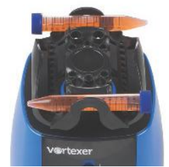
15 mL conical tubes x 2 (horizontally mounted)
