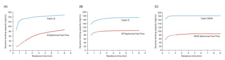
Fig 3. Dynamic binding capacity as a function of residence time for: (A) Capto Q and bovine serum albumin (BSA), (B) Capto S and α-chymotrypsin, (C) Capto DEAE and amyloglucosidase. For Sepharose Fast Flow resins, residence times below 2 min are not possible in large-scale columns.
