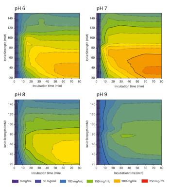
**Fig 10.** Screening for optimal binding conditions (pH, ionic strength and incubation time) for amyloglucosidase on Capto DEAE by batch uptake methodology using 96-well filter plates. Note that incubation time using this methodology is not equivalent to residence time in the column; typical residence times can be seen in Fig 2C.
