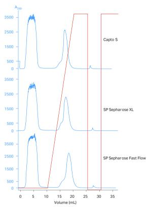
**Fig 6.** The separation ability of Capto S for  $\alpha$ -chymotrypsin compared to SP Sepharose Fast Flow and SP Sepharose XL resins in 1 mL prepacked HiTrap columns.
