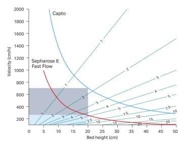
**Fig 4.** The highly rigid Capto base matrix allows a much larger window of operation (area below the curves) at large-scale than Sepharose 6 Fast Flow. This is particularly true at bed heights of 20–30 cm and above. Data correspond to a 1 m diameter column, at 20°C and viscosity of water. Red and blue curves correspond to pressure limits of 1.3 and 3 bar, respectively. Green contours give the residence time in the column in minutes.
