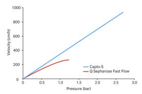
**Fig 2.** Pressure/flow curve for Capto S compared to Q Sepharose™ Fast Flow. Running conditions: AxiChrom™ 1000 for Capto S, Chromaflow™ 1000 for Q Sepharose Fast Flow, 20 cm packed bed, with water at  $20^{\circ}$ C. The pressure includes pressure drop from the bed and the column. System/tubing pressure is excluded.
