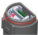
Figure 2: Push to unlock
