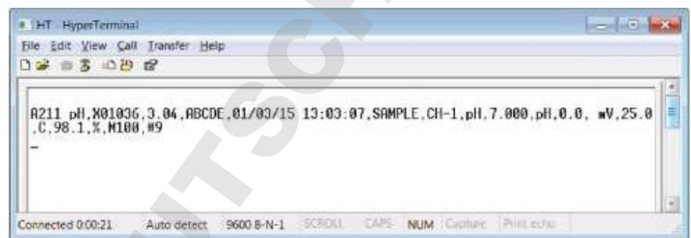
A screenshot of the HyperTerminal application window. The title bar says "HT - HyperTerminal". The menu bar includes "File", "Edit", "View", "Call", "Transfer", and "Help". The toolbar has icons for file operations. The main window displays a single data line: "R211 pH,X01036,3.04,ABCDE,01/03/15 13:00:07,SAMPLE,CH-1,pH,7.000,pH,0.0, mV,25.0,C,98.1%,M100,#9". Below the window, status bars show "Connected 0:00:21", "Auto detect 9600 8-N-1", and various keyboard indicator lights.
