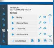
Customizable methods save electrode, titrant and sample titration settings so routine procedures can be repeated without additional setup or pre-work and methods can be shared among titrators using a USB flash drive.
