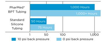
The performance of tubing in peristaltic pumping applications is affected by the conditions of use and equipment utilized, along with size and wall thickness of the tubing tested. The data above is presented for information only and should not be utilized for specification purposes.
