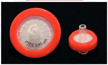
Naturally hydrophobic, the PTFE syringe filters are used for air sterilization or for the preparation of HPLC samples, for the filtration of solvents and corrosive solutions. For aqueous solution filtration, you need to wet the membrane with an adapted solvent such as ethanol or methanol.
