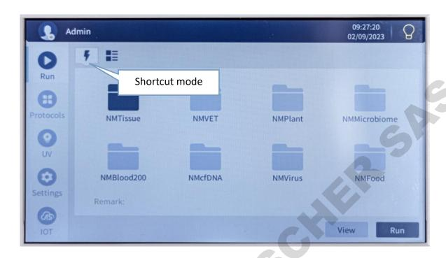
Under the shortcut mode, select the protocol needed and click "View". This will open the protocol view interface displaying information of protocol parameters of the individual steps. Clicking "Run", will run the protocol; clicking "Step run", will start the protocol from the selected step.
