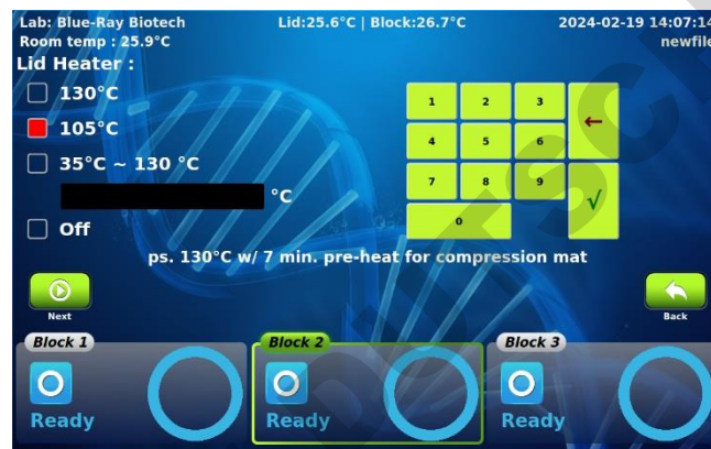
Figure 16. Lid heater control mode
