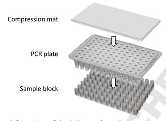
**4.** To prevent deformation of the PCR vessels, and to ensure even distribution of pressure from the lid, when PCR tubes or tube-strips are used, please load extra empty tubes into the 4 corner wells of the sample block. Always make sure that all the sample tubes/ tube—strips are distributed evenly over the sample block.
