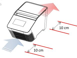
Please make sure there is no obstruction to the air flow around the unit. There should be at least 10 cm of free space at the front and back of the instrument.
