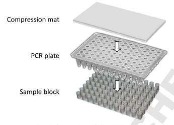
4. In order to prevent the deformation of the PCR vessels, and to ensure even distribution of the pressure from the lid, when PCR tubes or tube-strips are used, please load extra empty tubes on the 4 corners of the sample block. Always make sure that all the sample tubes/ tube-strips are distributed evenly on the sample block.
