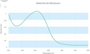
Absorbance values are certified at 260 nm, 280 nm and 330 nm for spectral bandwidths of 1.0, 2.0, 3.0, 4.0 and 5.0 nm . The value at 330 nm is used as a "background" correction, as in the normal methodology. From these values a corrected 260/280 ratio is calculated and reported for each bandwidth using the formula:
