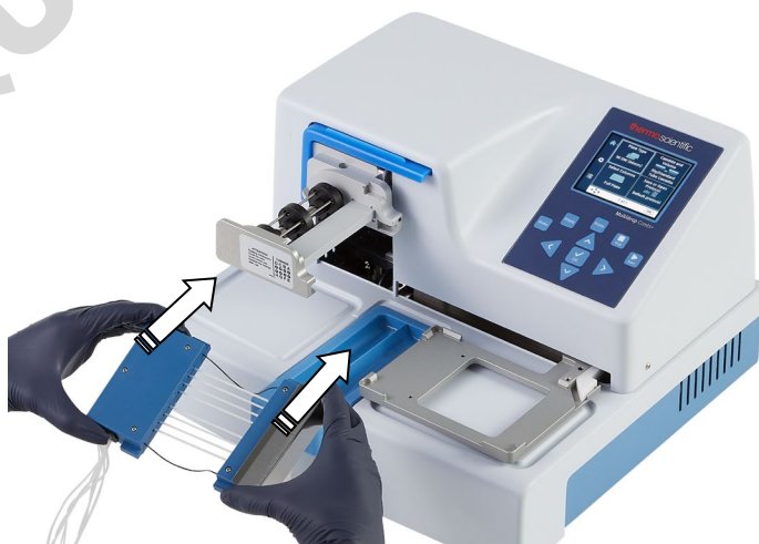
Figure 4-13. Insertion de la cassette de distribution
