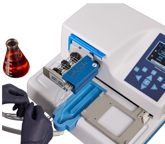
Figure 6–57. Cassette de distribution correctement installée
