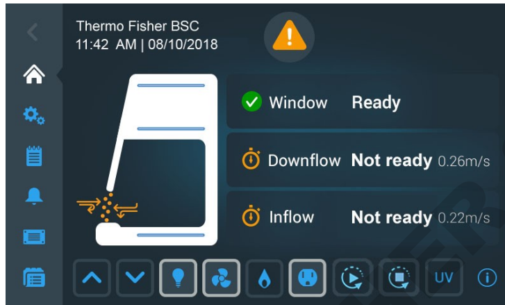
Figure 35 Main Screen - Unit starting up
