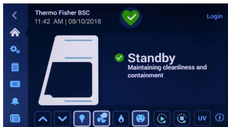
Figure 36 Main Screen - Unit in Standby
